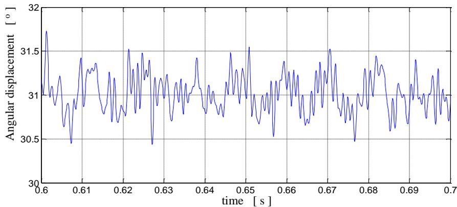
Fig 10. Chattering phenomenon - the results of the measurements.
