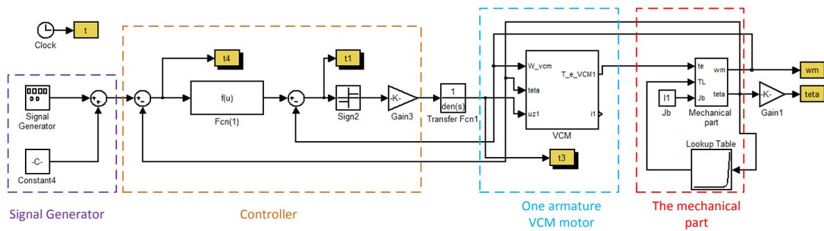
Figure 3. Implementation of time optimal control of exemplary single armature VCM motor
