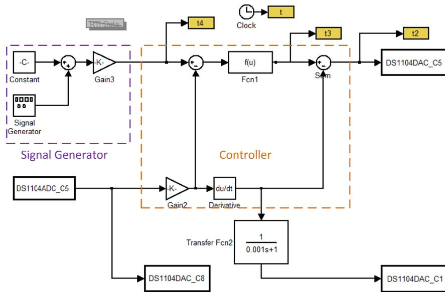
Figure 5. The controller of time optimal control implemented on the signal processor card dSpace 1104
