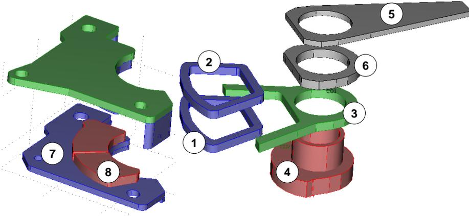
Figure 1. Geometry of two armature VCM motor and the rest of head positioning system components
