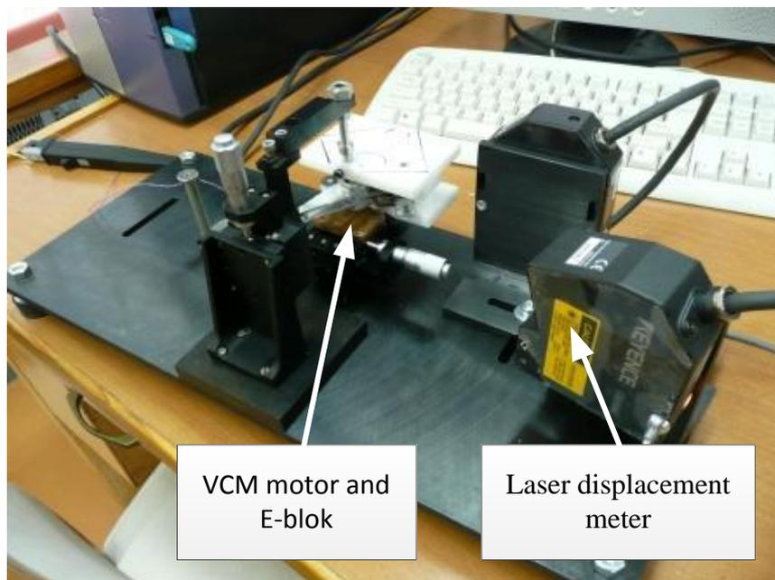
Figure 4. Test bench for investigations of VCM motor time optimal control
