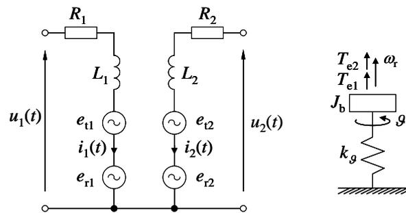
Figure 2. Circuit representation of two armature VCM motor [7]
