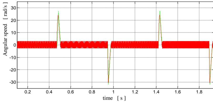
Fig 16. The angular velocity of the E-block - the results of simulation two armature VCM motor (red curve), and one armature VCM motor (green curve).
