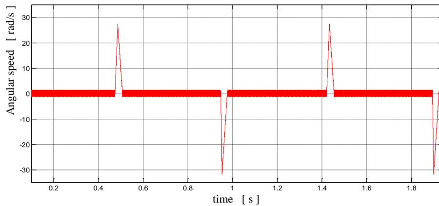
Fig 13. The angular velocity of the E-block - the results of simulation
