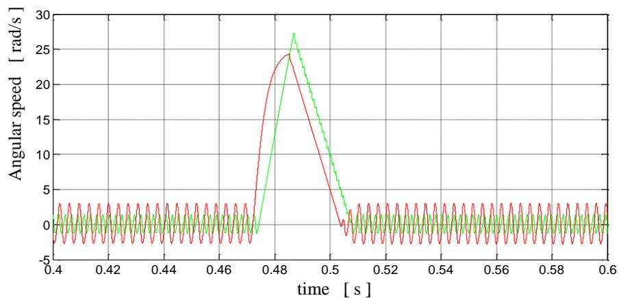
Fig 18. The angular velocity of the E-block - the results of simulation of two armature VCM motor (red curve), and one armature VCM motor (green curve)
