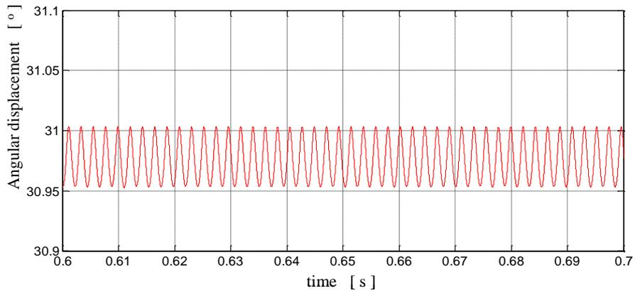
Fig 10. Chattering phenomenon - the results of the simulation
