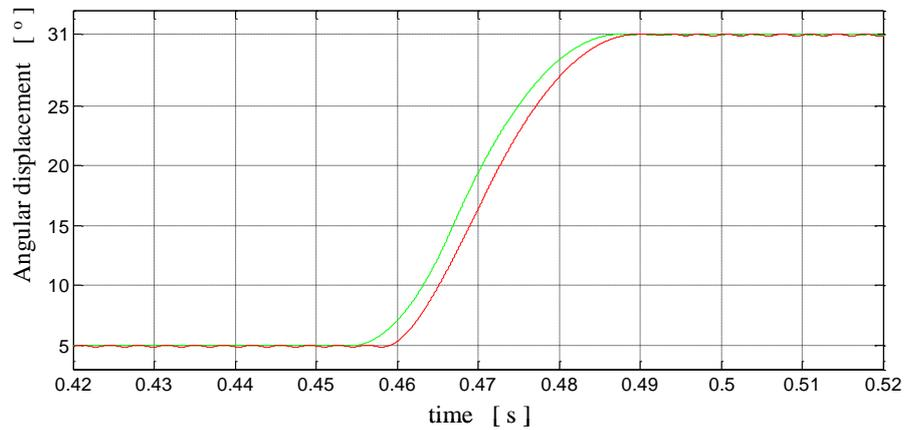
Fig 17. Angular displacement - the results of simulation of two armature VCM motor (red curve), and one armature VCM motor (green curve).
