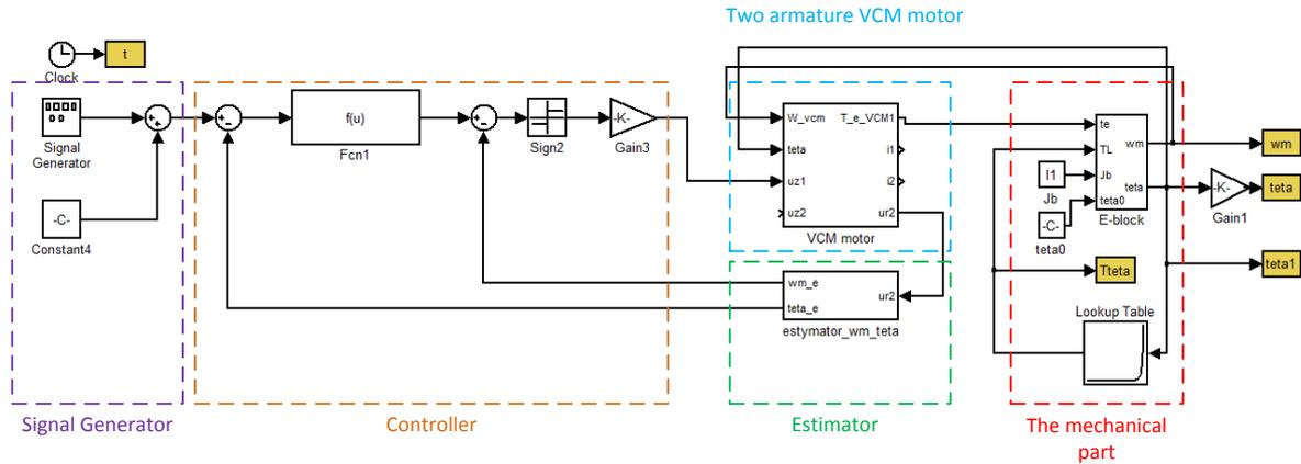
Fig 14. Implementation of time optimal control of two armature VCM motor
