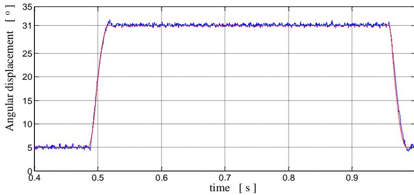
Fig 9. Comparison of the angular displacement the E-block. Blue waveform- results of measurement, the red waveform- result of simulation.
