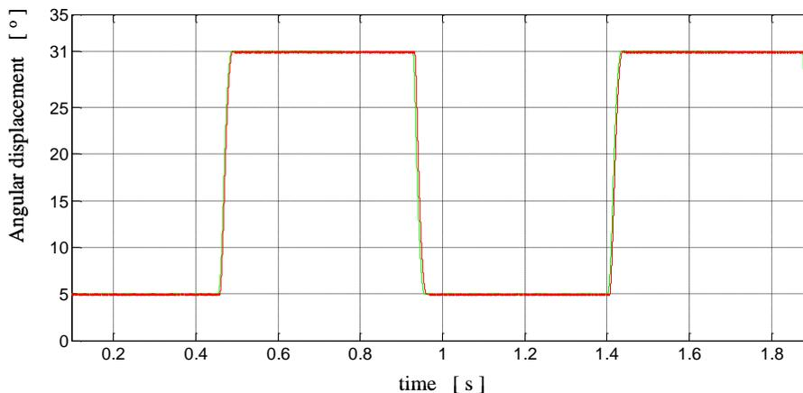
Fig 15. Angular displacement - the results of simulation two armature VCM motor (red curve), and one armature VCM motor (green curve)
