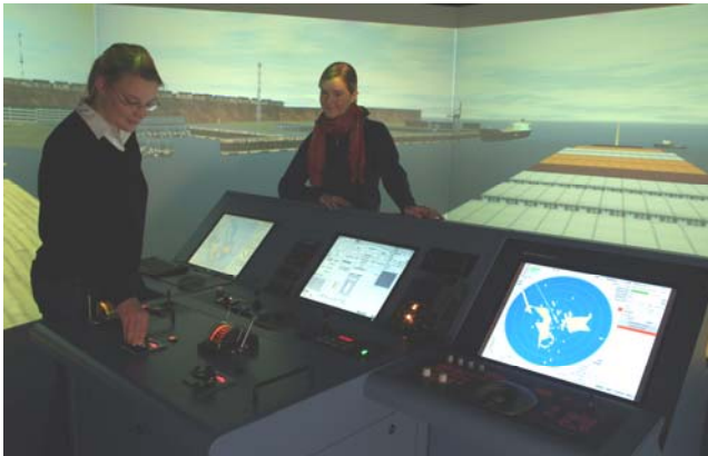
Fig. 4: Bridge 2 of Ship handling / Bridge Simulators with 260-degree visual display and NACOS (Radar, Conning and Track Radar) as well as handles for twin screw and twin rudder in exchange panel
