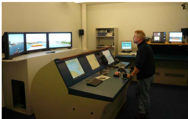
Fig. 5: Bridge 3 & 4 of Ship handling Bridge Simulators with 120-degree visual screen display and NACOS (Radar, Conning and Track Radar) as well as handles for twin screw and twin rudder and 2 Azipod Handles
