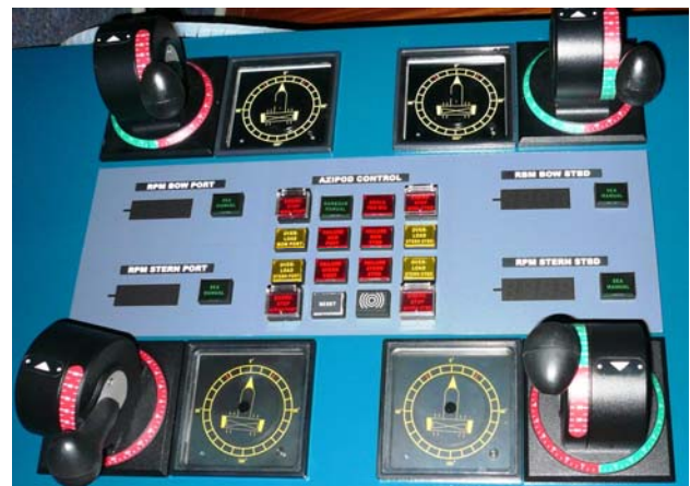
Fig. 3 Consoles with multiple steering handles 4 Azipod steering handles on exchange panels for bridges
