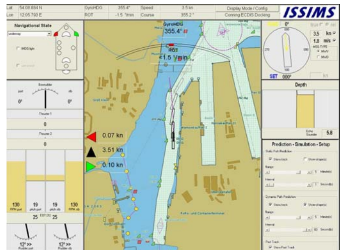
Fig. 11: Layout concept for Manoeuvring Prediction in ECDIS (left) with integrated presentation of different track predictions (centre) for rudder manoeuvres
