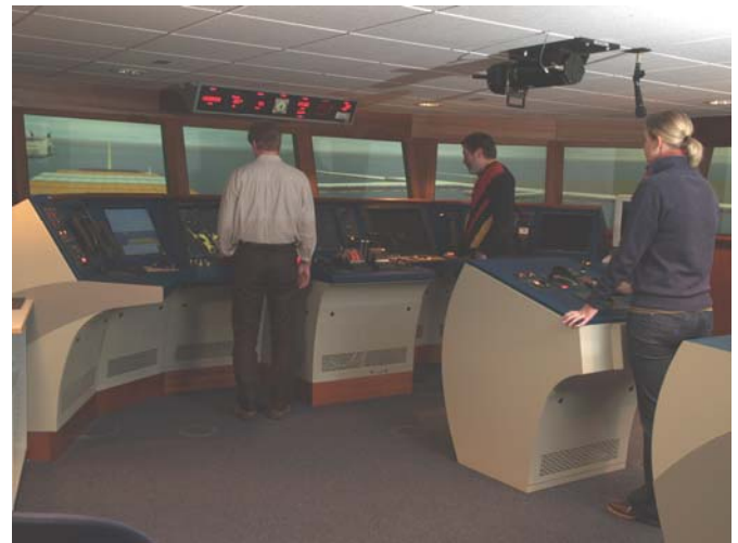
Fig. 2: Bridge 1 of Ship Handling Simulator with 360° projection system with full Integrated Bridge System NACOS and other features
