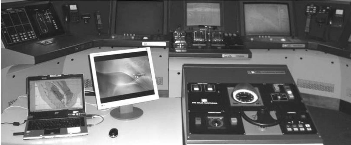
*Fig. 1: The additional trainings tool Manoeuvre Mate connected with the Ship Simulation System*
