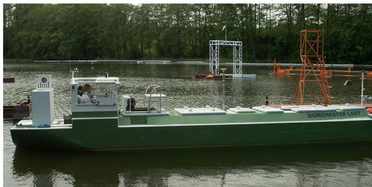
*Figure 1: Student Karina Wieseler from Wismar University on the bridge of the LNG tanker model during berthing manoeuvre at Ilawa Training Centre*
